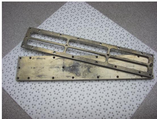
Fig. 1. Stainless steel holder designed to accommodate Kapton samples
